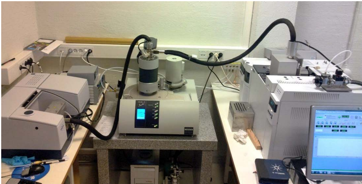
Figure 10. Simultaneous Thermal Analyzer (STA) device coupled to the Gas Chromatograph Mass Spectrometer (GC-MS) and to the Fourier Transform Infrared Spectrometer (FT-IR) used for the measurements of chemical composition of samples.
