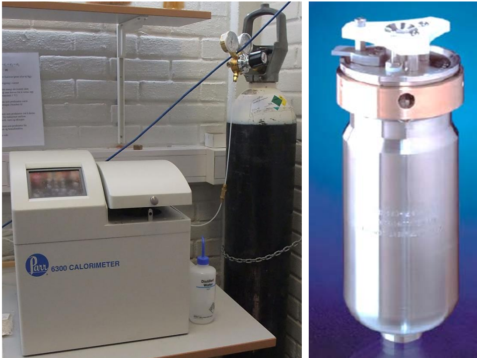
Figure 11. Automatic Isoperibol Calorimeter 6300 (left) and its oxygen combustion bomb (right) used for the calorific value measurements.
