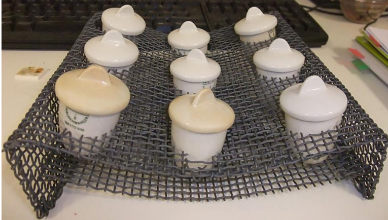
Figure 12. Porcelain crucibles filled with grinded samples of stem wood, stem bark, branch wood and twigs used for the ash content measurements.
