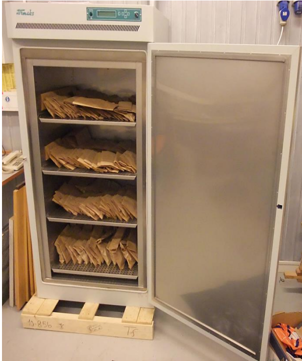
Figure 9. Termaks drying oven used for the moisture content measurements of samples.
