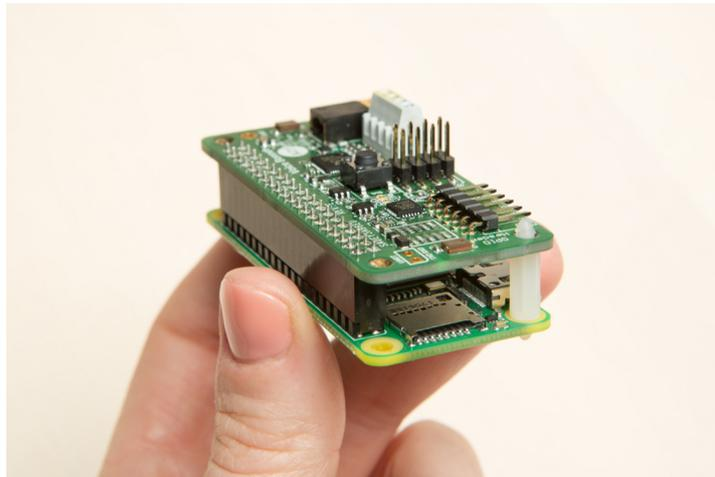
Figure 8.4: Google Voice Kit: A Voice Bonnet board that has the same Myriad 2 processor as in NCS is placed on top of a Raspberry Pi Zero.
