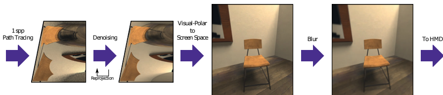
Figure 4.4 An example of a path tracing and denoising rendering pipeline using Visual-Polar [P5]
