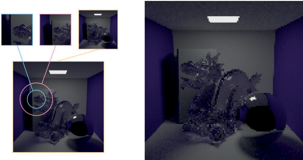
Figure 4.1 An example image of how multiple resolution foveated rendering can be done. The left side shows the relative sizes of the three renderings and how the frame is constructed. The right side visualizes the sample coverage by using nearest neighbor interpolation in upsampling the lower quality renderings.
