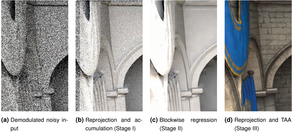
Figure 3.8 The results of different BMFR pipeline stages. Here the camera is rotating leftwards. Therefore, leftmost pixels can use only current frame data in the reprojections and TAA on stages I and III.
