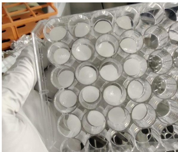
Figure 22. 11mm diameter cylinder-shaped samples fit perfectly in 48 well plates
