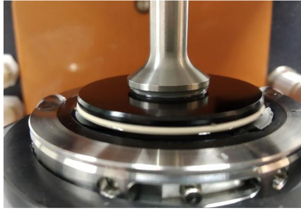
Figure 15. Two-plate system with 20 mm diameter plate geometry
