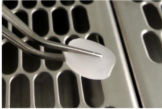
Figure 20. Hybrid sample for cell cultures, diameter 11 mm, height 3mm
