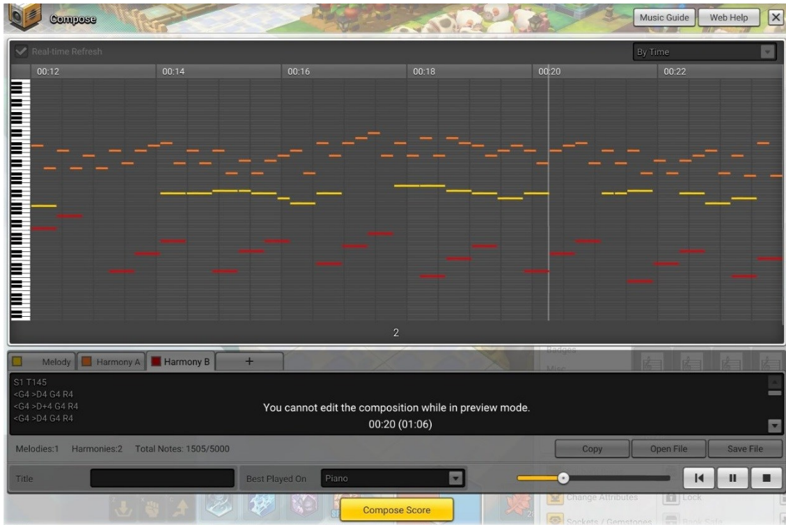
Figure 7. The composer interface with code displayed at the bottom. Whitespace is ignored by the interface and notes are here arranged on multiple lines for improved readability.
