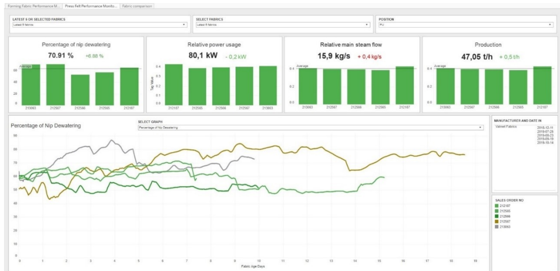
Figure 12. PMC Analytics - Performance monitoring dashboard. Benchmarking tool for user to compare fabric's performance
