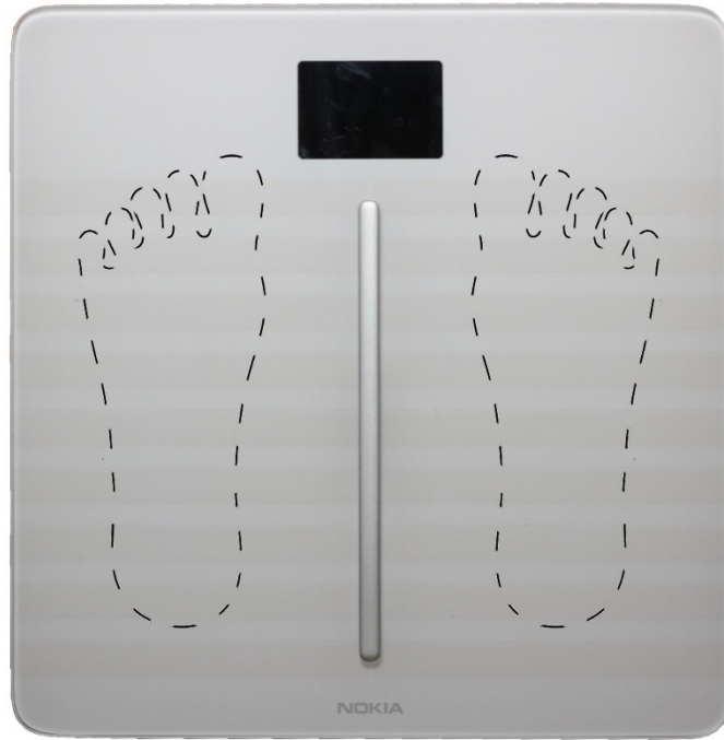
Figure 6. An edited photograph of the Body Cardio smart scale that displays the optimal placement of feet for measurements. The horizontal bands are the electrodes on the surface of the scale. The user should stand on the scale with bare feet so that their heels are on top of the second horizontal electrode.
