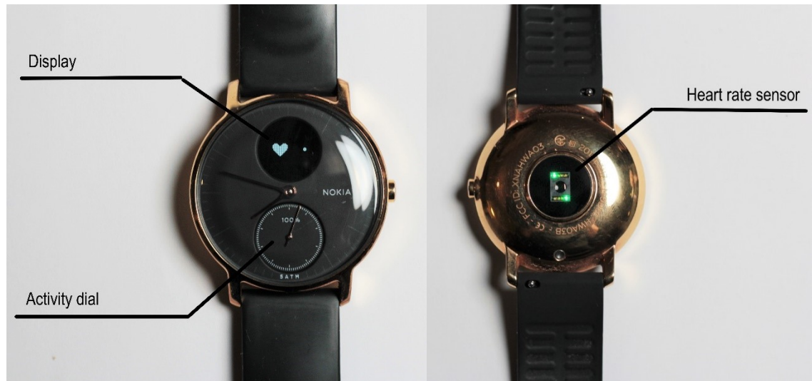
Figure 5. Photographs of the Steel HR watch that show the different components of the watch. The watch includes an analogue watch, a digital display, and an activity dial in the front, and a HR sensor in the back.
