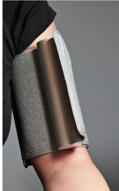
Figure 7. The Nokia BPM+ is placed around the upper arm approximately 2 cm above the elbow.
