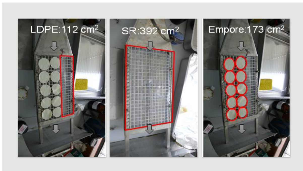
Figure 1 Co-deployed AlteSil™ silicone rubber (SR sampler) and SDB-RPS Empore disks (ED sampler) and LDPE stripes (LDPE sampler) in a DPS device. The arrows show the direction of water streaming through the exposure chamber.
