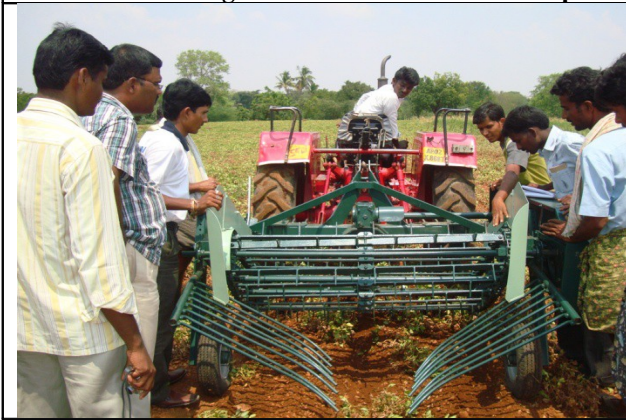
Groundnut harvesting with digger, shaker cum windrower
