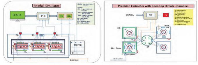
Fig. 3.5: Process flow diagrams for data acquisition through PLC in SCADA for Rainfall Simulator and Precision Lysimeters
