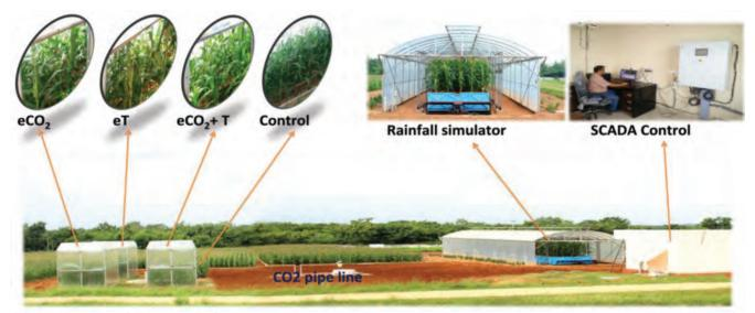
SCADA based rainfall simulation facility and Precision type lysimeters with open type climate chambers was also established for assessing the climate change impact on resource losses in CCRC, Hayathnagar.
