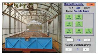
Calibration of nozzles and SCADA screen
