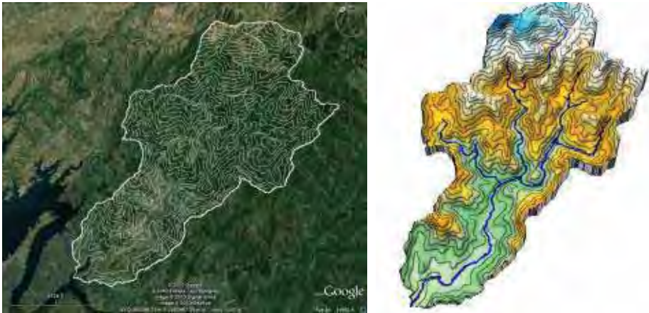
Figure 5. GIS (free open source) delineated contours derived from ASTER data draped in Google earth and a 3D DEM derived from it. (Prepared by D R Sena as an example).
