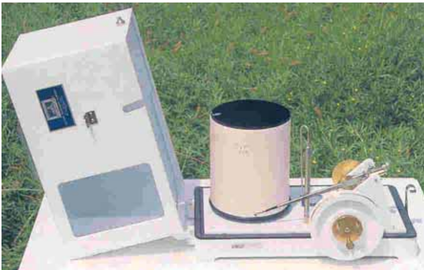
Figure 8. A drum-type mechanical runoff recorder.
