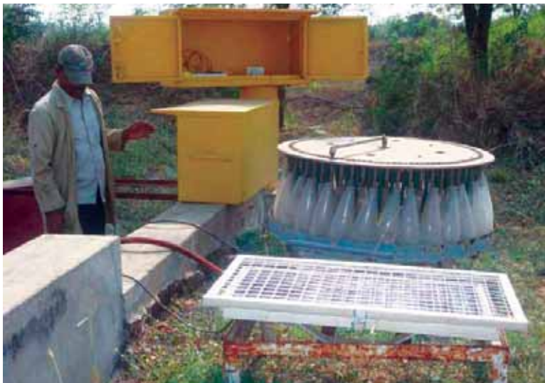
Figure 10. Integrated digital runoff recorder and sediment sampler device (new microprocessor is shown in inset).
