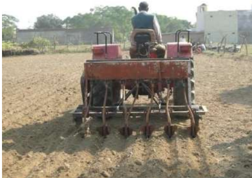
Seed cum Fertilizer Drill sowing of wheat Drill sowing of rainfed wheat
