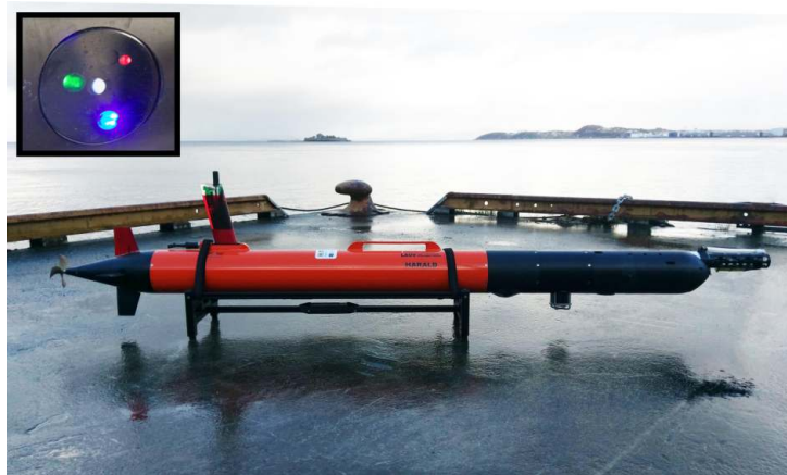
Figure S.1: LAUV Platform. NTNU's Light AUV platform ( Harald ) for upper water-column exploration used in our work. The onboard EcoPuck sensor ([Chl a ], [cDOM], and [TSM]) is shown as mounted on the AUV in the upper left corner.
