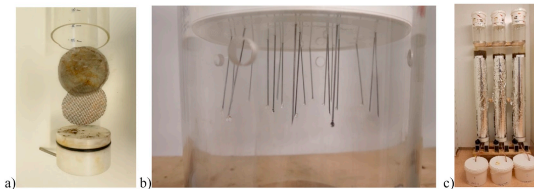
Fig. 1. a)The coarse and fine filter at the bottom of the columns; b)The top water reservoir with 25 needles to distribute the infiltration; c)The column set up.
