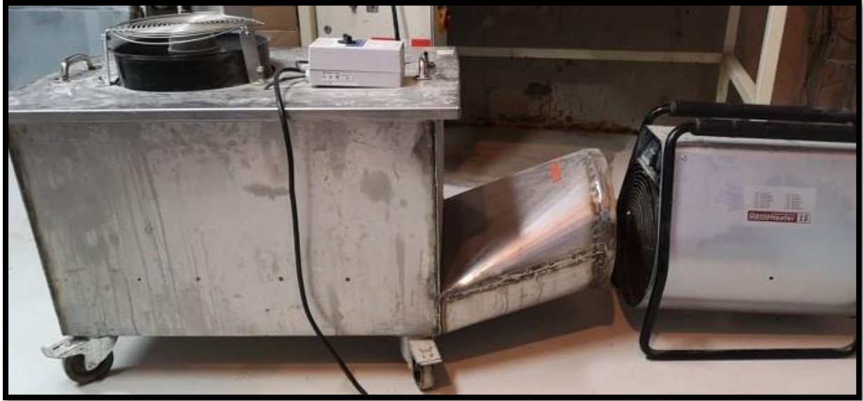
Figure 3-2 - From left to right, Picture of the batch drier with an outward blowing fan lid, Fan heater in front blowing hot air (15KW) into the batch drier (operating position).
