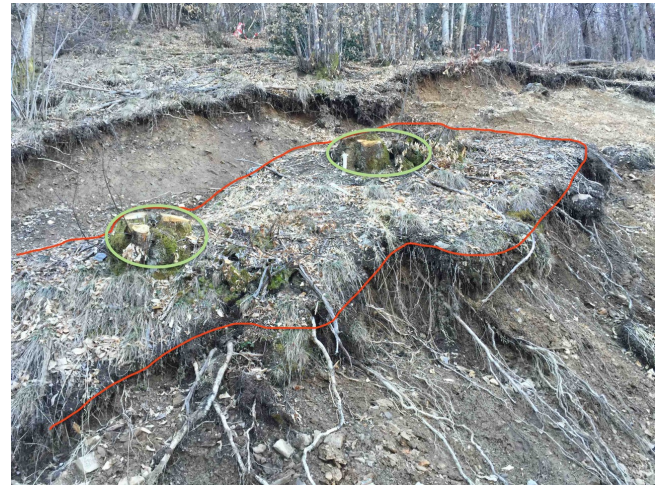
Figure 12. Example of a weak zone in a forested area showing isolated tree stumps with a root system that behaved as a stiff island during the opening of a gap in a weak zone in between root systems of adjacent trees.
