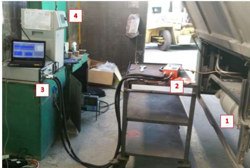
Figure 2: Experimental setup: 1: DPF; 2: 379020A-30 Thermodiluter Head; 3: 379020A-30 Thermal Conditioner Air Supply; 4: EEPS 3090
