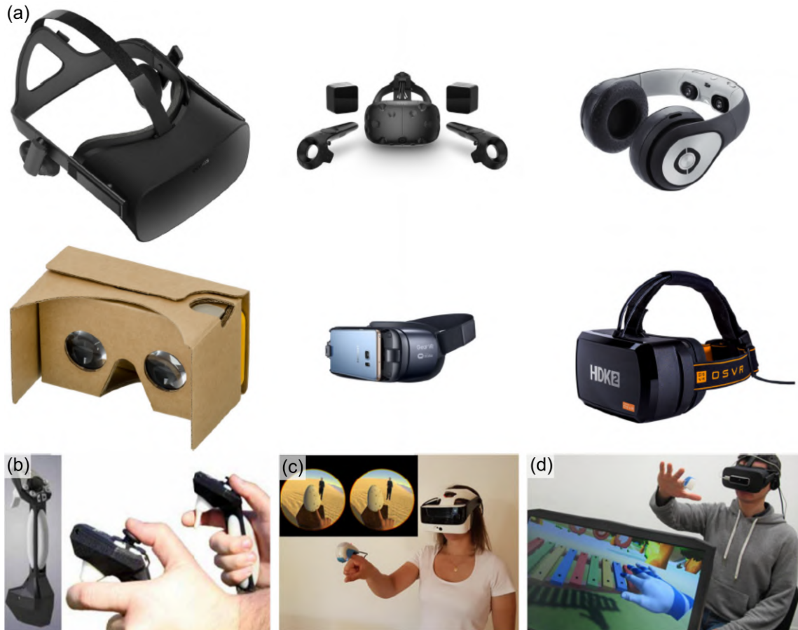
Figure 2.12: The new era of VR devices and haptics. (a) Modern head-mounted displays. Top row from left to right: Oculus Rift, Steam VR/HTC Vive, and Avegant Glyph, bottom row: Google Cardboard, Samsung Gear VR and OSVR HDK. Image taken from. 158 (b) Reactive Grip Motion Controller by Tactical haptics. This device includes tangential motion and skin stretching capabilities to recreate the grip sensation in VR environments. (c) The Tactai Touch™ system by Tactai. This system acts on the fingertips of the user to mimic the sensations of pressure or texture during VR interactions (d) The VR touch system by GoTouchVR. It operates similarly to the Tactai Touch, using vibrating actuators to stimulate the skin. Pictures (b) to (d) are taken from. 163
