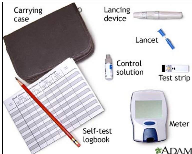
Figure 1.1: Standard Diabetic Glucose Monitoring Equipment including diagnostic meter, lancet for piercing skin and test strip for collecting blood and transporting it to the diagnostic meter [2]
