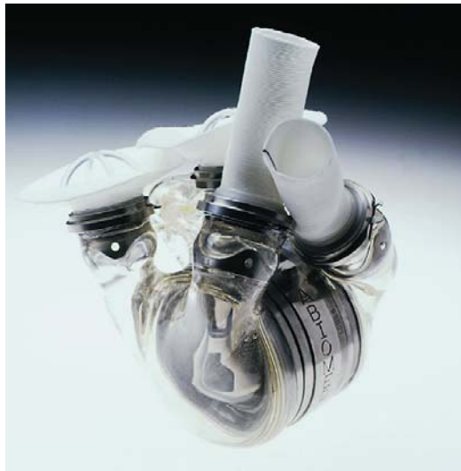
Figure 1.2: The AbioCor implantable replacement heart uses an implanted electronics package to monitor and control pumping speed of the heart based on the physiological needs of the patient [5].
