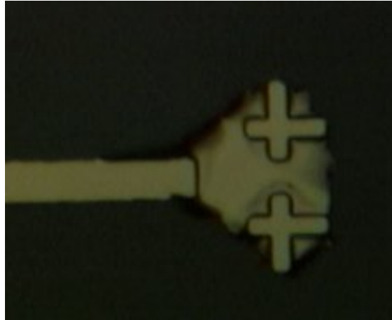
Figure 6.4: 0.25 \mu\text{m} thick gold coil trace with excess gold remaining between the trace and the small alignment marks.
