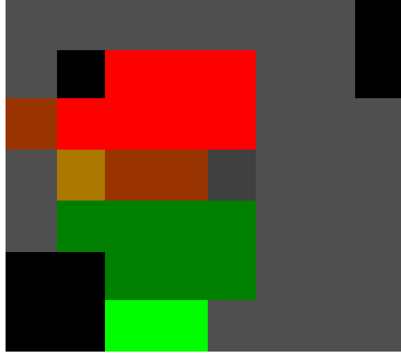
Figure 3.4: The data processor forms an HSI chip using a track’s predicted position and uncertainty. The chip shown here consists of two vehicles (one red and one green) and is an example of a fused chip, where the bounded regions for the two tracks overlap. The black rectangular regions (lower left and upper right) are outside of the region of interest and no data are associated with them. The chip, therefore, can be non-rectangular in shape.
