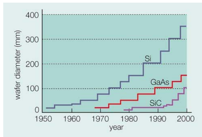
Figure 17: The increase in wafer diameter as a function of time, demonstrated for R&D GaAs, Si and SiC wafers. SiC wafers have gone from 25 to 100 mm in about half the time it took GaAs or Si to make the same increase [22]
