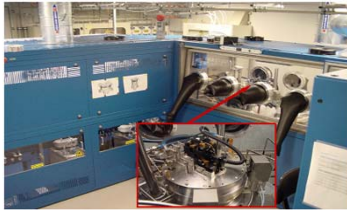
Figure 12: GaN MOCVD Reactor System [15]
