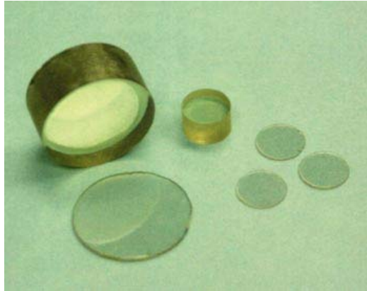
Figure 18: ZnO boules and wafers. ZnO is being developed as a material suitable for GaN epitaxy [22].
