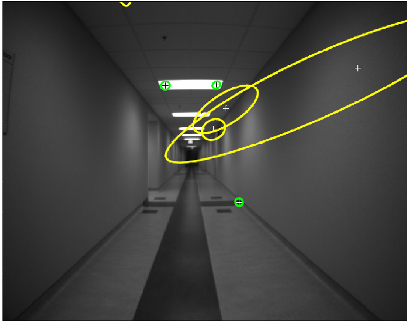
Figure 4.2: Sample image from indoor data collection. The indoor data collection presents the filter with man-made features in an office environment. The crosses and ellipses indicate the locations and uncertainty of currently tracked landmarks [28].
