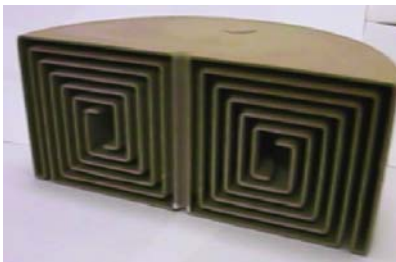
Figure 19: Stanford’s “Swiss Roll” burner concept to be used in conjunction with a thermoelectric generator [53].
