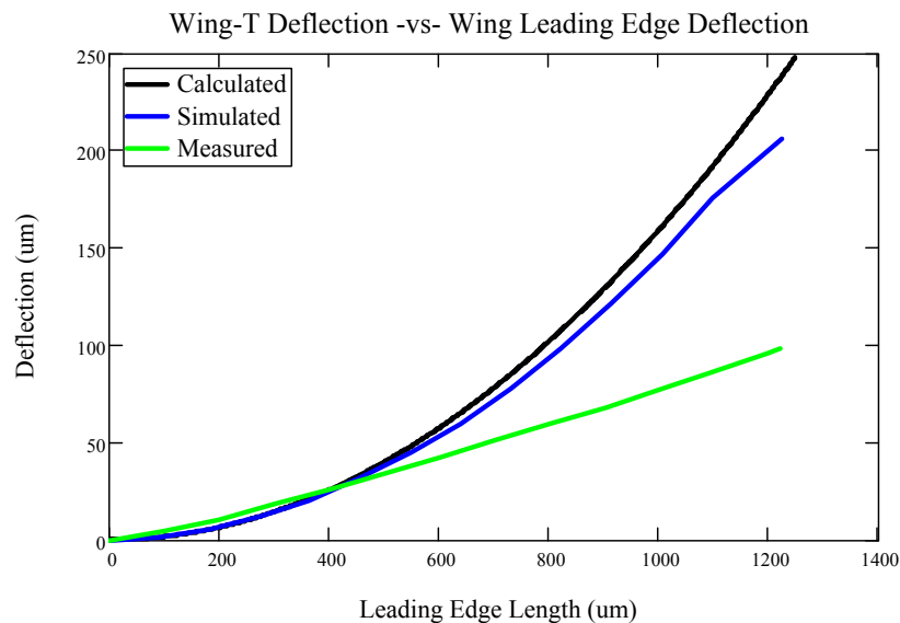
Figure 76: Wing-T empirical data compared to calculated and simulated deflection. The measured data closely resembles calculated and modeled data up to 0.5 mm.
