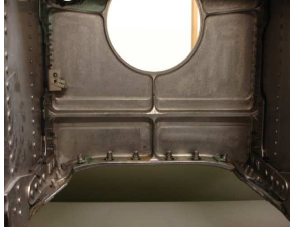
Figure 1.1: USAF aircraft bulkhead known to suffer fatigue cracks [7]
