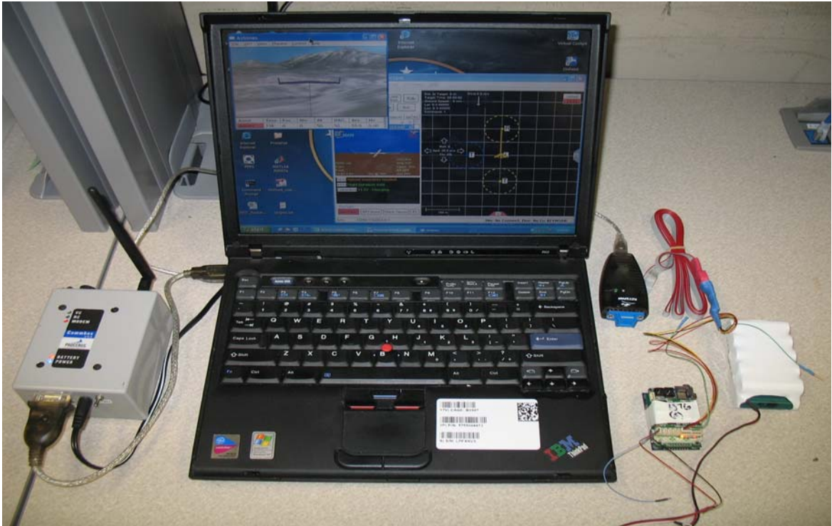
Figure 34. Representative HIL setup
