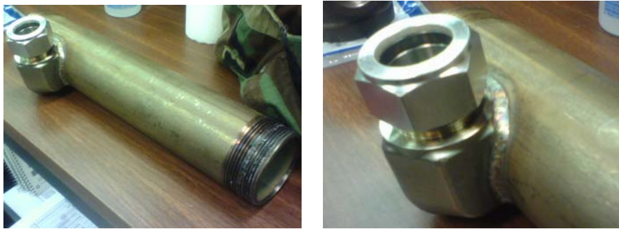
Figure 21. Union point of crossover tube and secondary detonation tube
