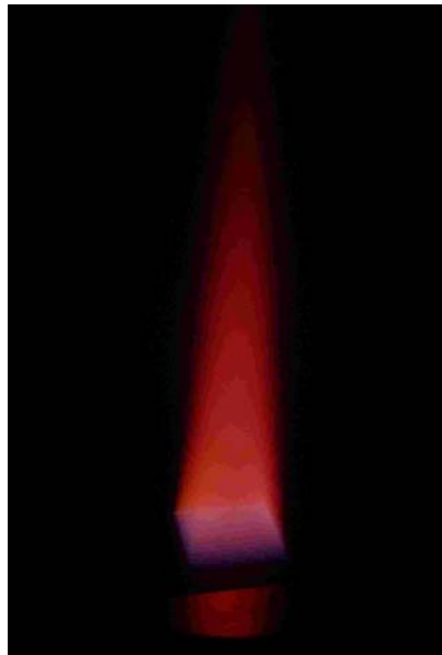
Fig. 6. Laminar Flame Produce by a Hencken Burner (photo by Chris Zickafoose)
