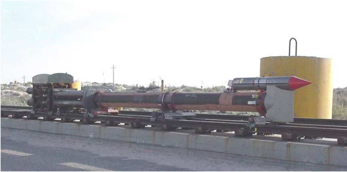
Figure 1.1: A test sled train on the HHSTT.
