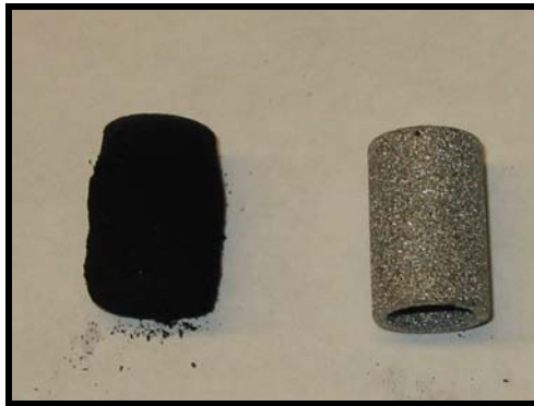
Figure 30. Photograph of coke covered filter after testing next to a filter without coking
