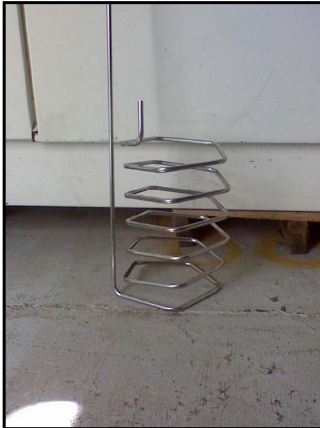
Figure A.1. Coiled type 316 stainless steel 3/8 in. tubing used in fuel cooling system
