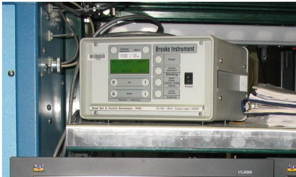
Figure 40. Mass flow controller for cooling hole air/N 2 flow
