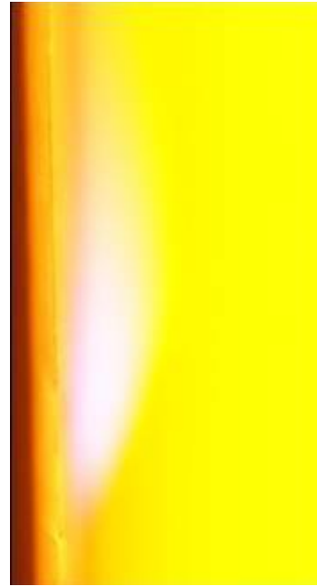
Figure 52. Visible combustion in cooling film, angled holes, M = 2.0
