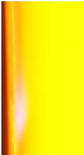
Figure 53. Visible combustion in cooling film, angled holes, M = 1.0
