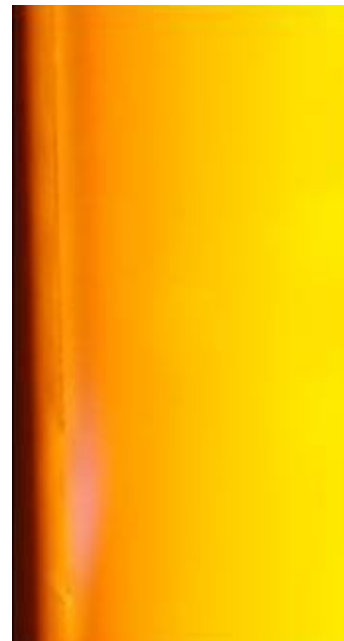
Figure 54. Visible combustion in cooling film, angled holes, M = 0.5
