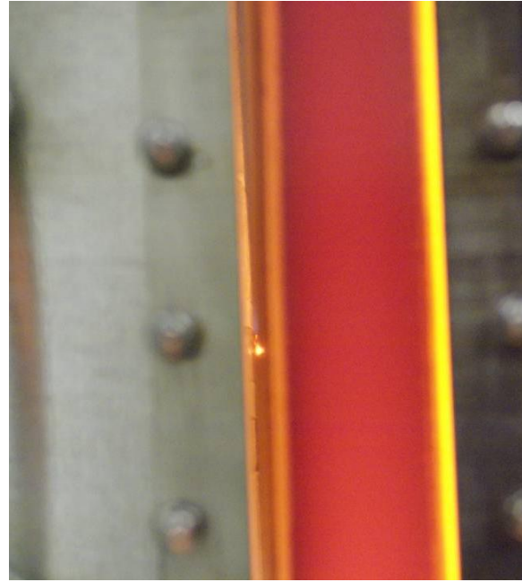
Figure 50. Visible combustion in cooling film, normal holes, M = 0.5
