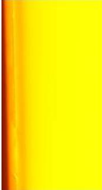
Figure 51. Nitrogen cooling film, angled holes, M = 2.0
