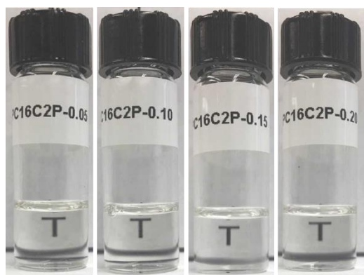
Figure 3.20. Optical images of dispersions of PC16C2P-0.05, -0.10, -0.15, and -0.20 in PAO at a concentration of 1 wt% at room temperature.
