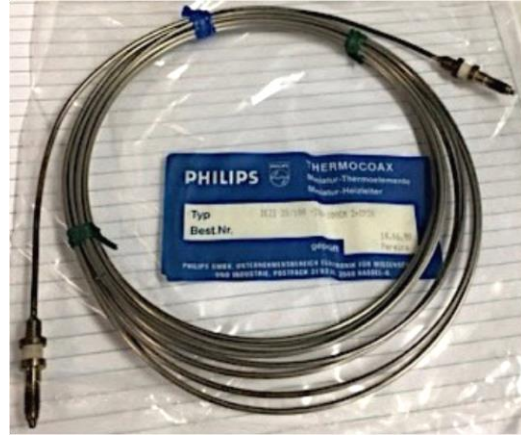
Figure 3.7. Images of self-heating target plate (left) and example of Thermocoax resistive heating cable (right).
