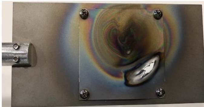
Figure 3.10. Picture of new SS target plate with thin SS insert plate after plasma exposure (left). Significant damage and discoloration are apparent. Schematic of thick SS insert plate with gridded holes also shown (right).
