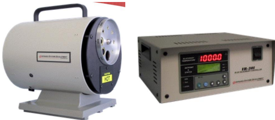
Figure 3.2. Images of IR-564 Black Body Radiation Source (left) and 301 Digital Temperature Controller (right).
