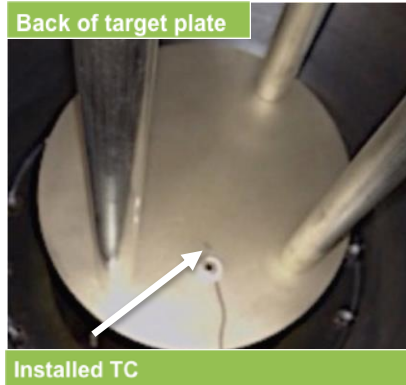
Figure 3.5. Non-plasma facing (left) and plasma facing (right) sides of the thin SS target plates. White arrows point out installed thermocouple locations. Surface damage due to plasma exposure is apparent on plasma-facing side (right).
