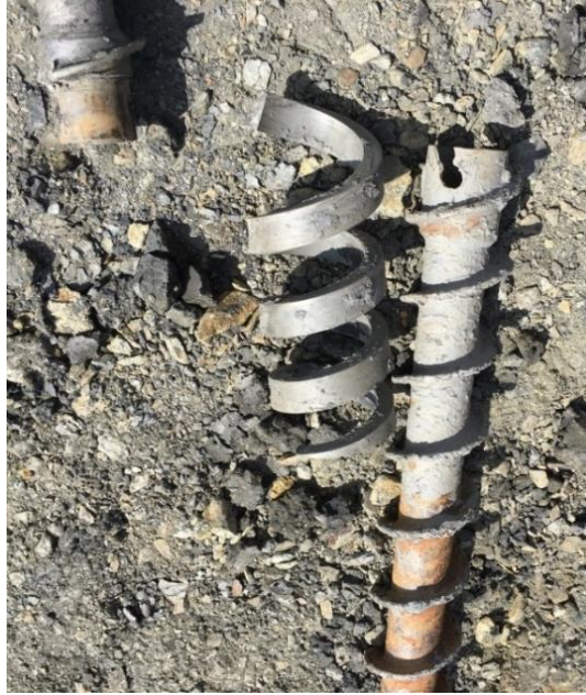
Figure 3-5. Broken Auger Recovery Tool Resulting from Attempted Recovery of Broken Auger. Total Depth of Augers in the Ground at the Time of the Break was 44 m; Auger Breakage (Segment at Right) Occurred at about 5m.
