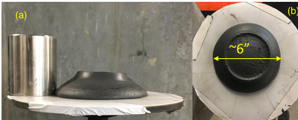
Figure 6-3. FCR specimen at the end of the flow table test indicated by the specimen edge reaching the 6" diameter mark. (a) side view (b) plan view
