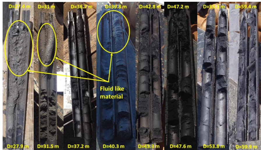
Figure 5-4. Observation of "Fluid-Like" material in in situ samples
