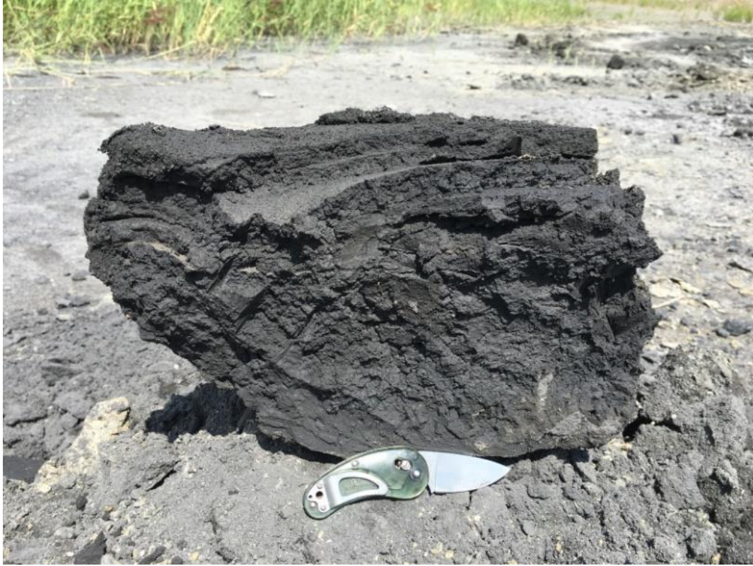
Figure 3-4. Bulk Sample Obtained from Approximately D = 5 m when a Track hoe was required to Extract a Broken Auger. The Knife Included for Scale has a Length of Approximately 250 mm (5 inches).
