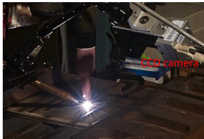
Figure 23. Passive vision weld pool image acquisition system
