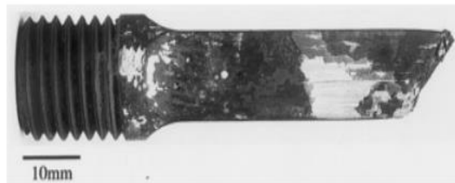
Figure 2.1: Photograph showing typical low-ductility 2.25Cr-1Mo/ In-82 interface failure observed in simulated creep tests at 590-625°C, stress<80MPa [14]
