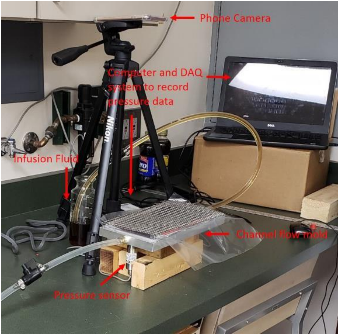
Figure 26: System for measuring in plane permeability of fabric through the channel flow mold technique
