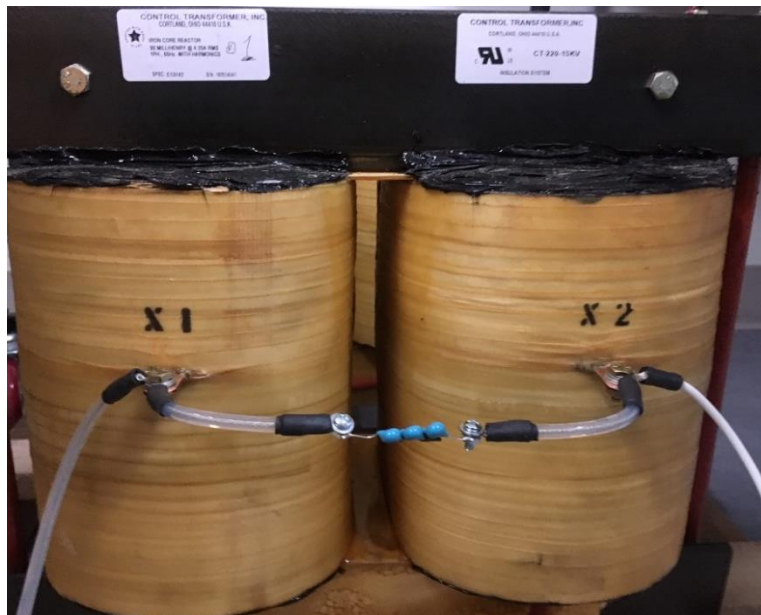
Fig. 34. High voltage load inductor with external capacitor to increase its EPC.
