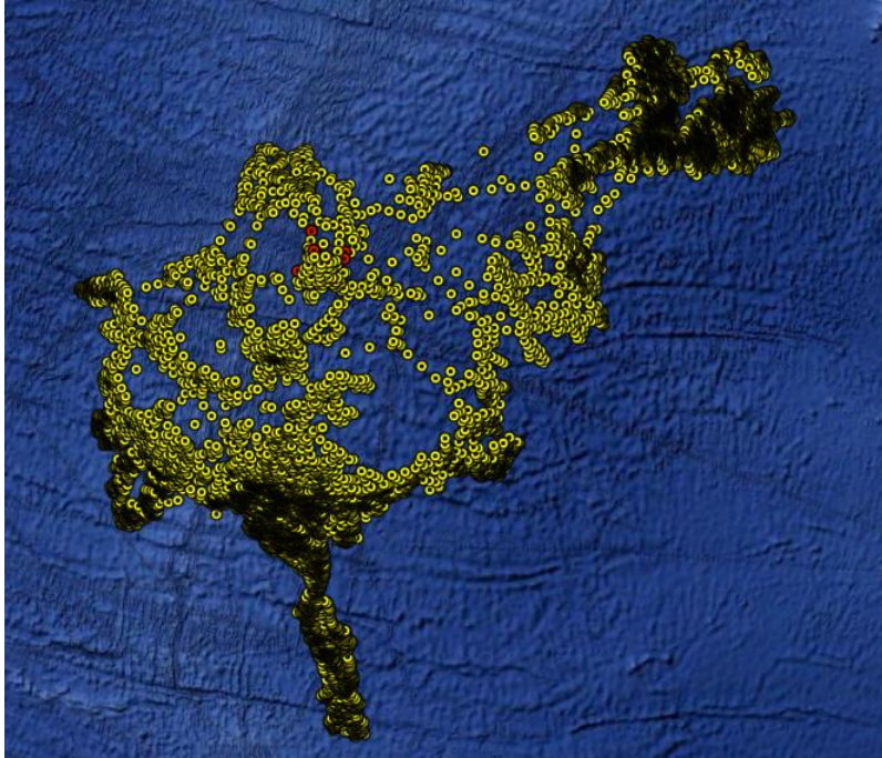
Figure 4.26. Google Earth image of entire Atlantis 9000 system buses (yellow) and buses tripped in Stage 2 (red) from tripping largest load in Zone 14
