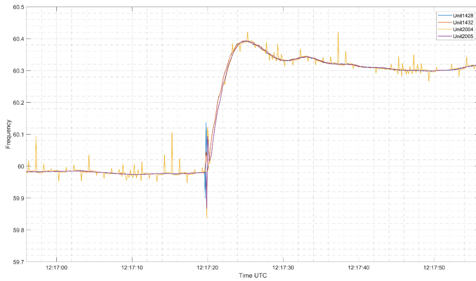
Figure 3.35. Frequency measured by UGAs during fast frequency ramp up or possible load drop detected on 09/03/2018 at 12:17:20 UTC
