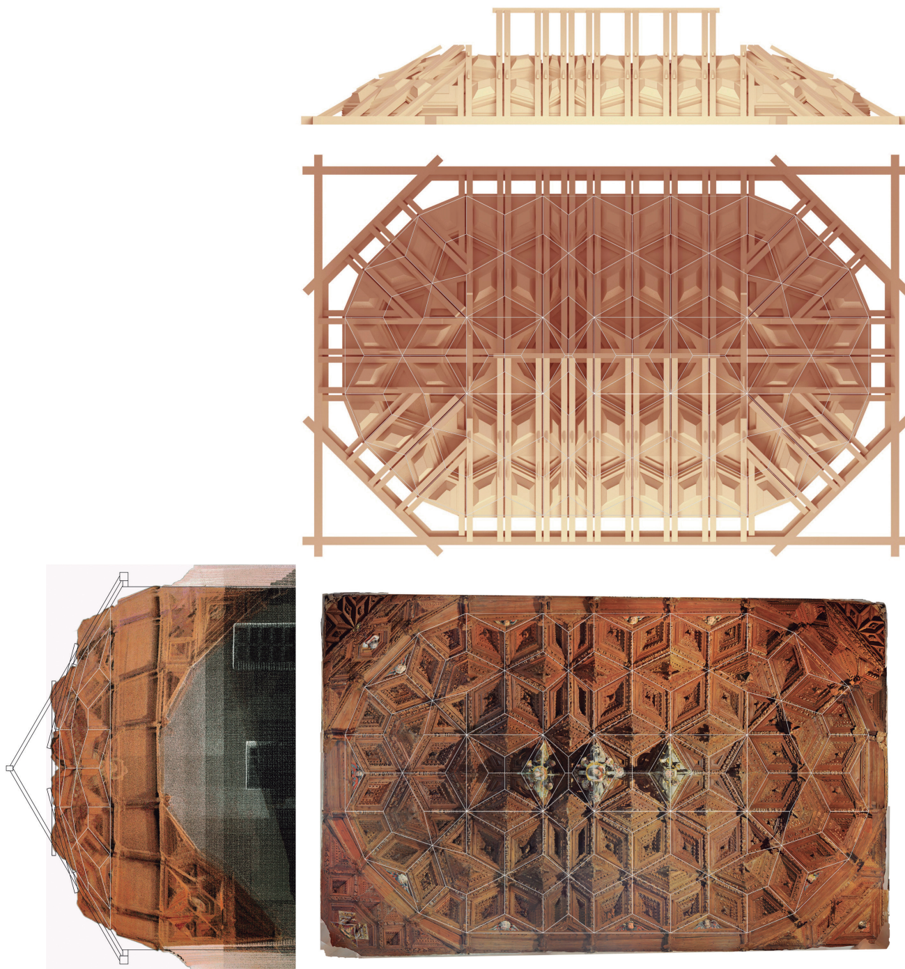
Figure 6. Above, front and top views of the structural system with concave and convex coffers. Below, right and bottom ortographic projections of the ceiling in its actual state, prepared by means of laser scanning and automated photogrammetry. The regularity of the coffered ceiling, compared with the deformations in the walls, frieze and pendentives, seems to confirm the rigidity of the coffered set and the validity of the analysis.
