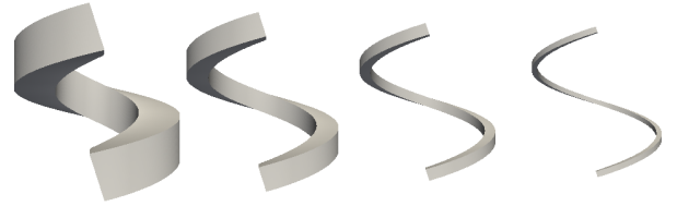
FIGURE 5. Helicoidal spring geometry for different thickness/length ratios: 0.1, 0.05, 0.025, 0.0125.
