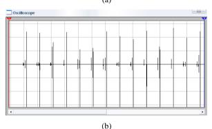
Fig. 9. (a) Zero Crossing Detector Circuit Output Signal, (b) Discharging Process of The Capacitor
