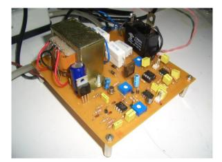
Fig.5. Capacitive Discharge Circuit Implementation.
