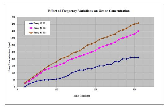
Fig. 12. Effect of Frequency Variation on Ozone Output
