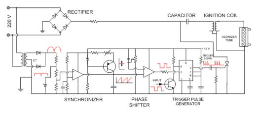
Fig.1 Capacitive Discharge Circuit For Ozone Generator
