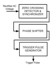
Fig.3. Zero Crossing Detector Block Diagram
