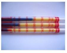
Fig.11. Ozone Output Measured by the Colorimetric Method.
