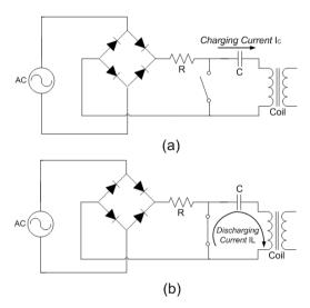
Fig.2. (a) Charging Cycle and (b) Discharging Cycle
