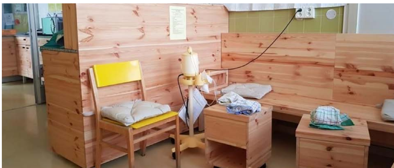
Figure 8.15: Reconstructed waiting zone in foyer of pavilion M in National Onological Institute in Bratislava made for demonstration and testing the application of wood in health care facilities, there is used pine and larch without finishing, design: Veronika Kotradyová, Martin Boleš, photo: Noro Knap
