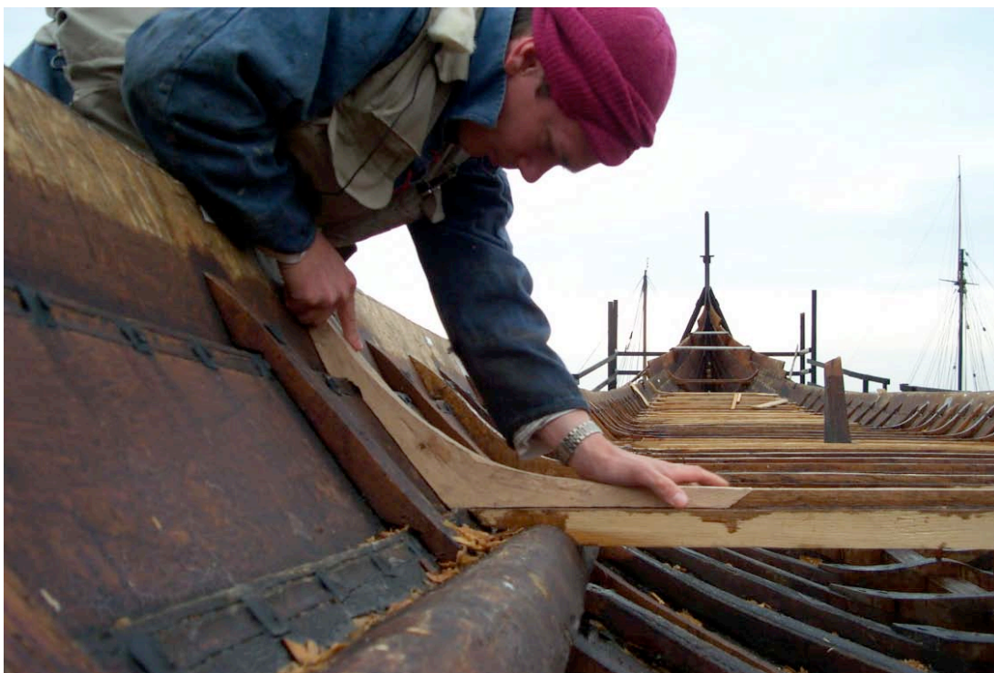
Fig. 10 Viking ship upper deck knee made by the author under instruction from Birger Andersen at the Roskilde Viking Ship Museum, 2003.
