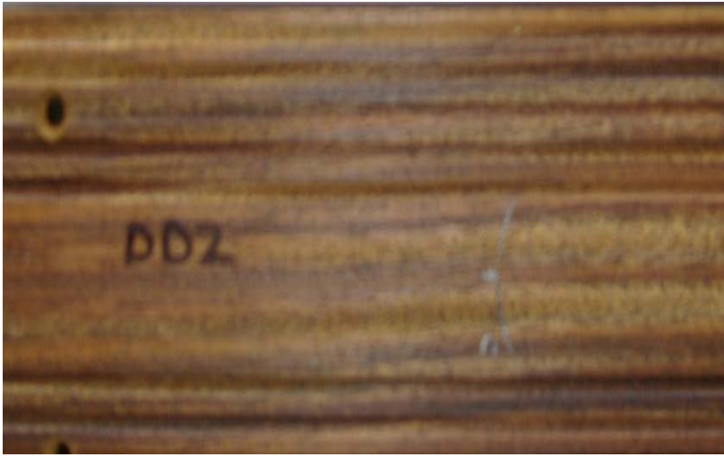
Figure 4.19 Denya heartwood planned unexposed.
