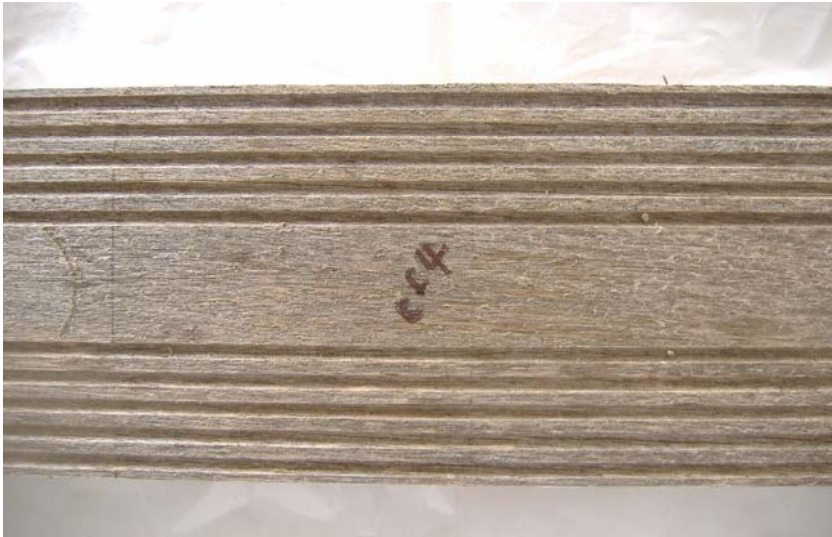
Figure 4.18 Esa treated with deck oil and exposed for six months out of doors.
