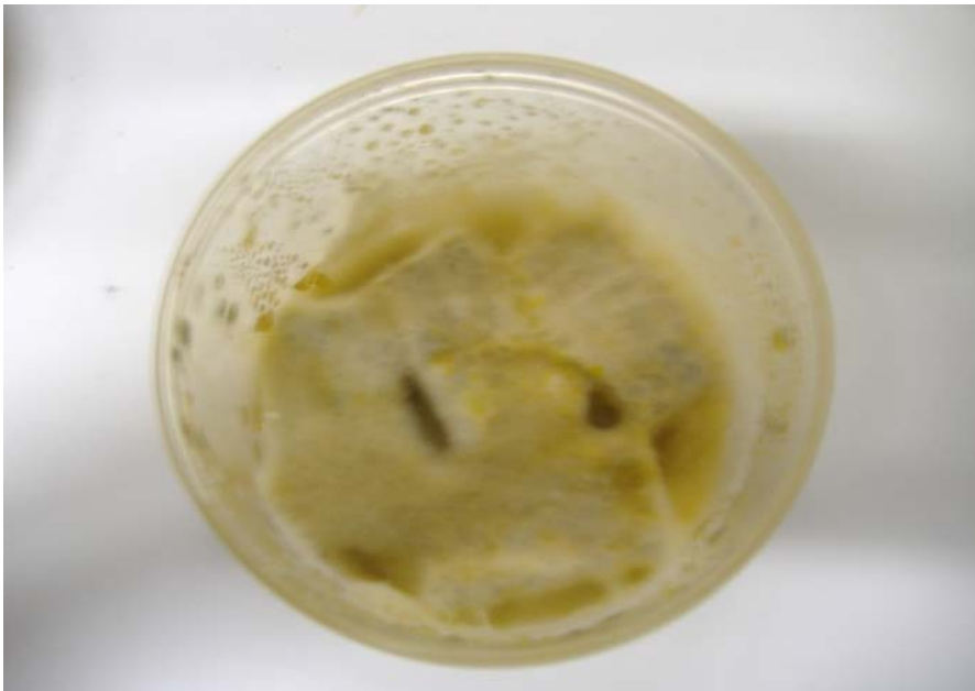
Figure 5.2 Mycelium covering wood specimen
