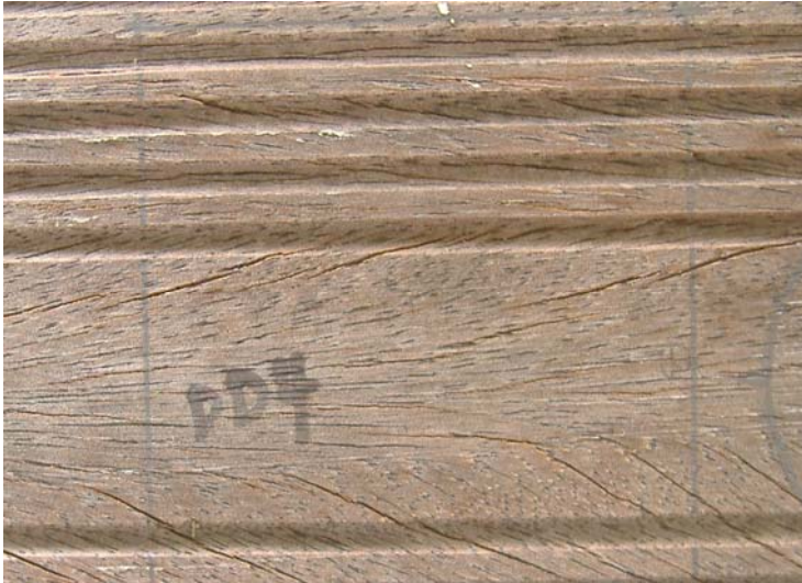
Figure 4.46 Exposed face of a denya sapwood board with checks in December 2006
