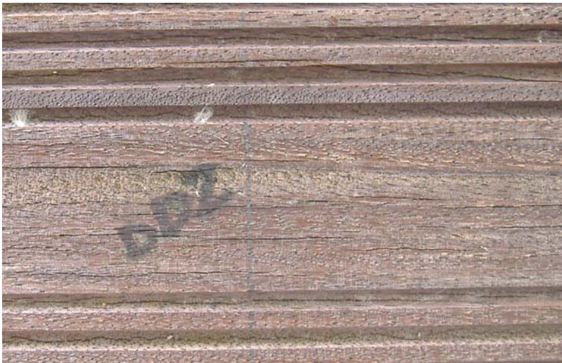
Figure 4.20 Denya heartwood planned exposed out of doors for six months.
