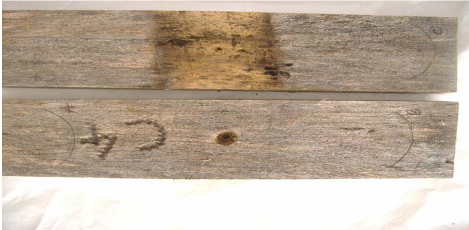
Figure 4.50 Stain on the surfaces of untreated esa cross pieces.
