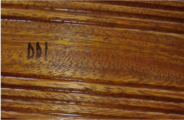
Figure 4.25 Denya sapwood treated with decking oil unexposed.
