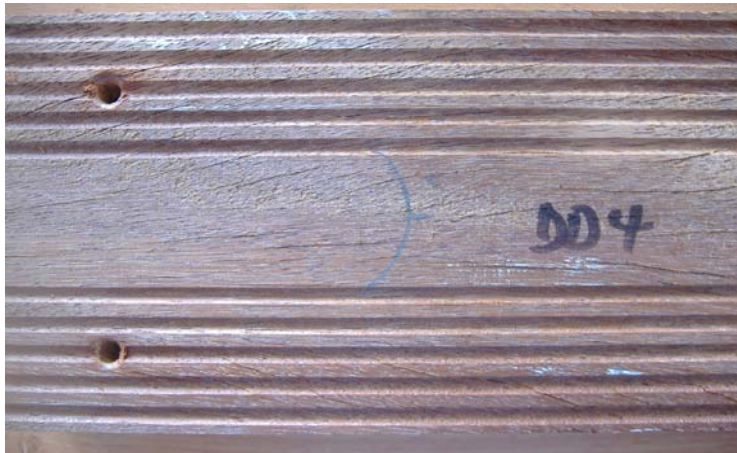
Figure 4.45 shows the surfaces of a denya decking board with checks in September 2006.
