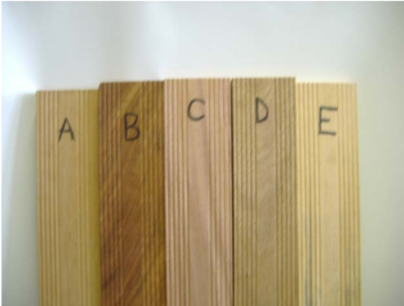
Figure 7.4 Untreated and unexposed decking boards included in the survey.
