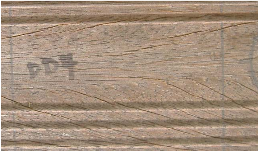
Figure 4.24 Untreated denya sapwood exposed out of doors for six months.
