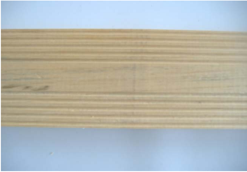
Figure 4.17 Esa treated with deck oil unexposed.
