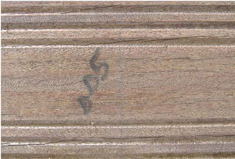
Figure 4.22 Denya heartwood treated with decking oil weathered out of doors for six months.
