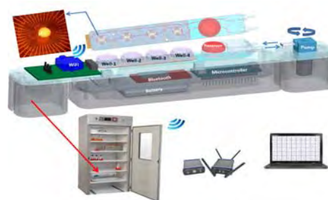
Fig. 1. Complete system: MEA chip, wifi system, perfusion pump.
