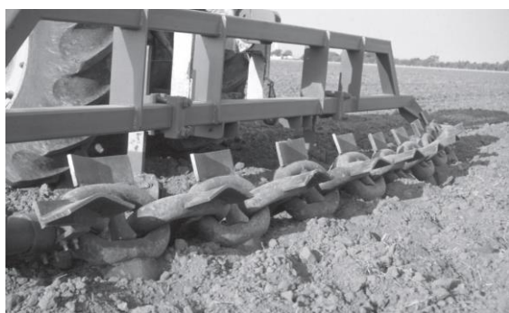
Fig.4 a) Machine that produces holes on the surface of the processed soil by rotating a chain with pallets b) The appearance of the land after passing the machine [1]
