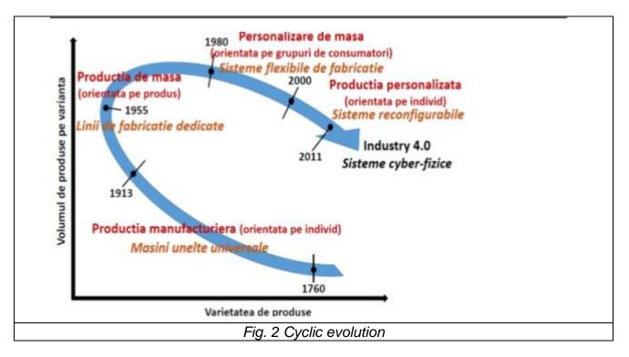
From Fig. 2 it follows that this concept has undergone a cyclical evolution, from personalized (individual-oriented) craft research to mass production (productoriented), then to personalized massproduction (consumer-oriented) and returning back to personalized production. (focused on the individual consumer).
