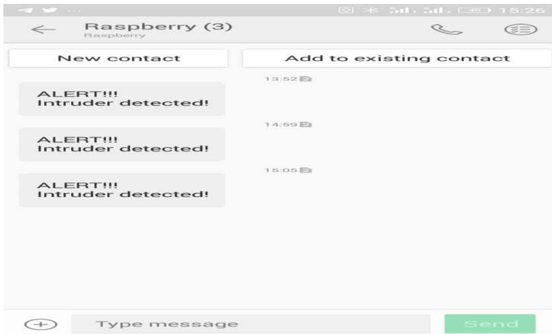
Figure 20: The SMS received after the raspberry Pi sent the mail.
