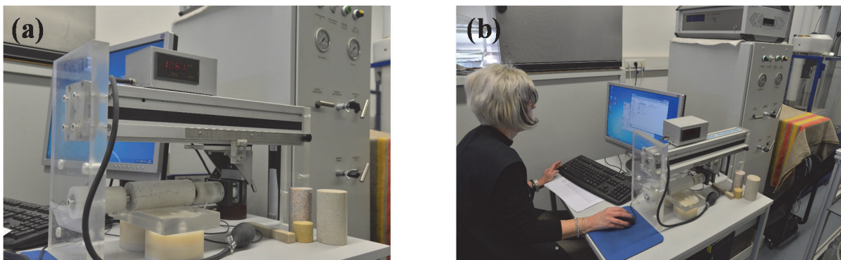
Figure 3.2 (a) ultrasonic wave speed measurement (b) data acquisition
