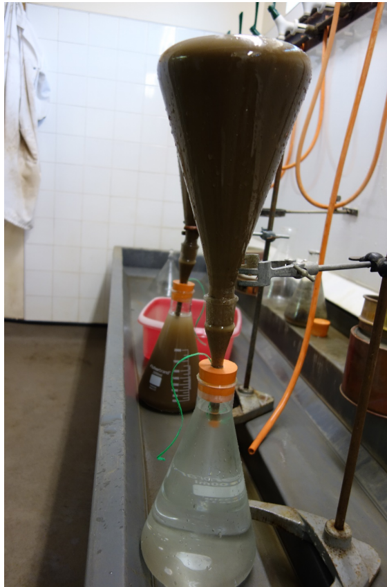
Figure 2.3. Seinhorst two-flask method showing the sedimentation process. (Courtesy, Nasamu Musa, Harper Adams University)
