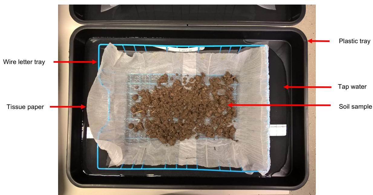
Figure 2.2. Setup for the Whitehead nematode extraction method. The technique depends on the nematodes' active migration towards a higher moisture gradient.
